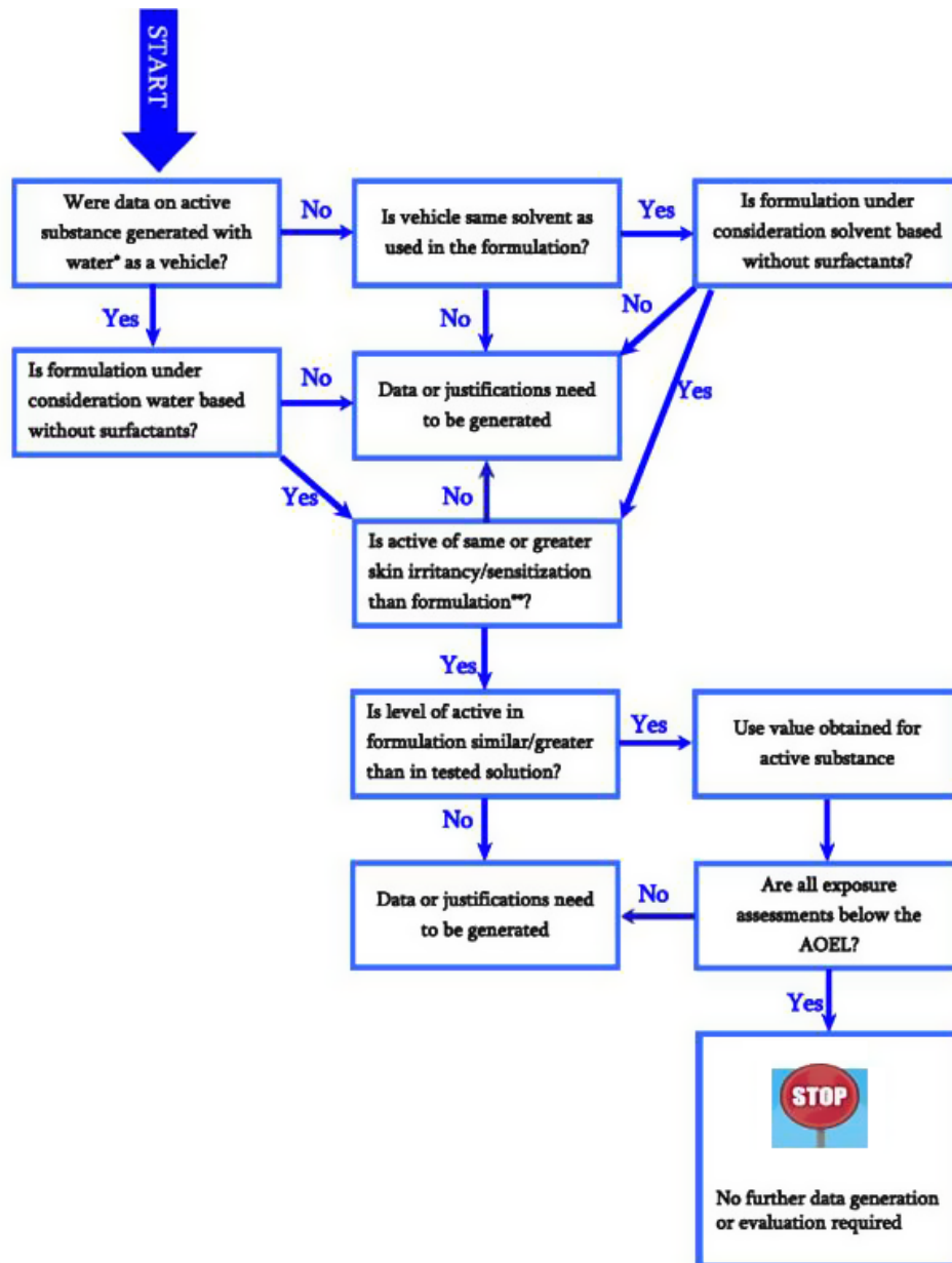
Flow chart 6: Procedures to follow when extrapolating dermal absorption data on an active substance to a formulated product
